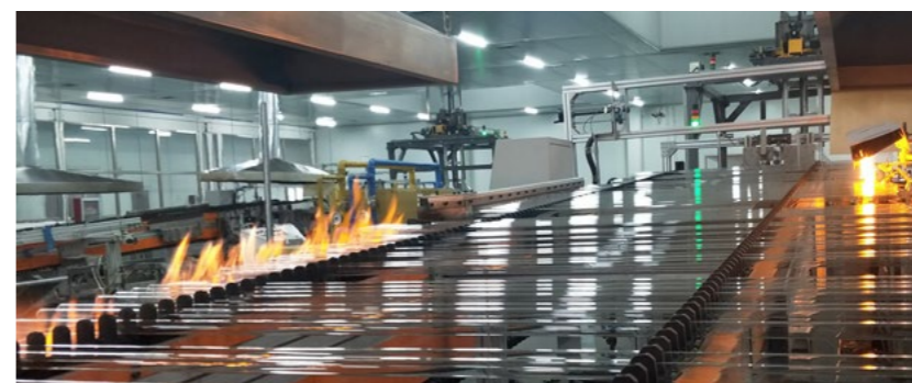
Production line of neutral borosilicate pharmaceutical glass tubes in Triumph Science & Technology
