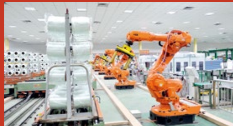
▼ The robotic arms on a tank-kiln wire drawing assembly line of Jushi Group
