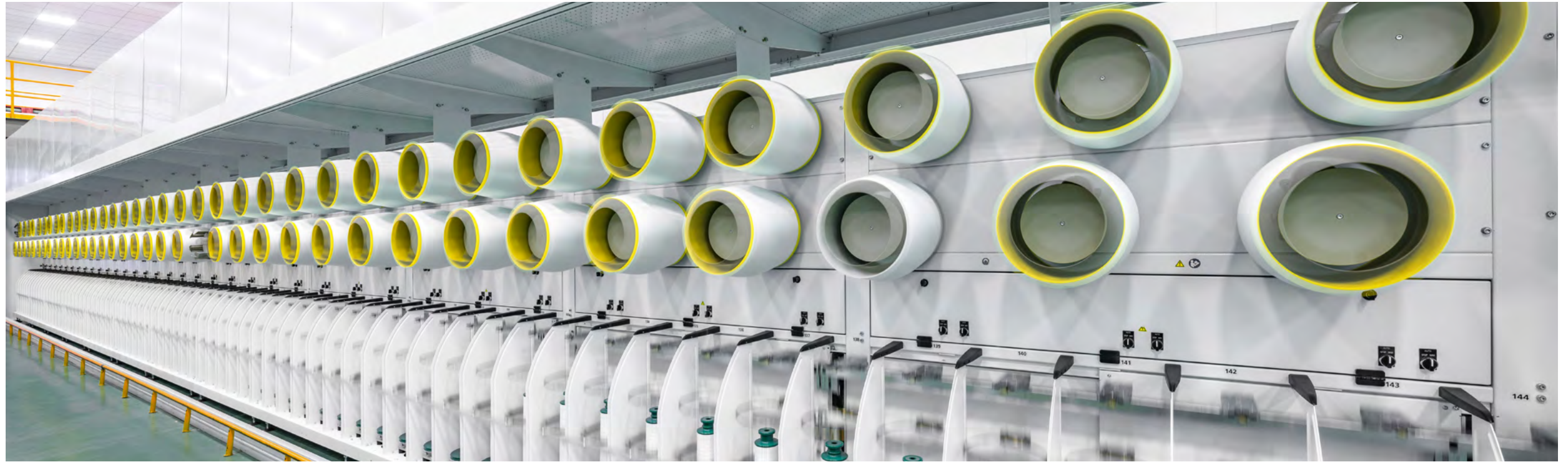
China Jushi's Twisting Workshop of Electronic Fabric Production Line with an Annual Output of 300 Million Meters
