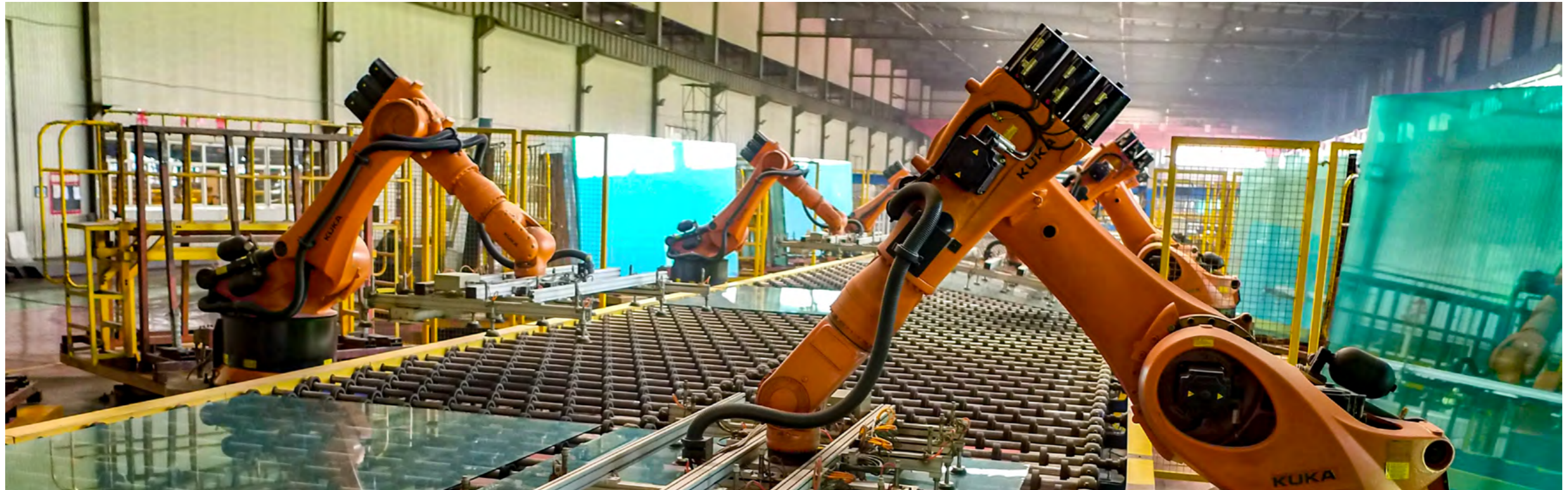
© CNBM Triumph Robot (Shanghai) Co., Ltd. - Flat glass production line cold-end hierarchical stacker robot
